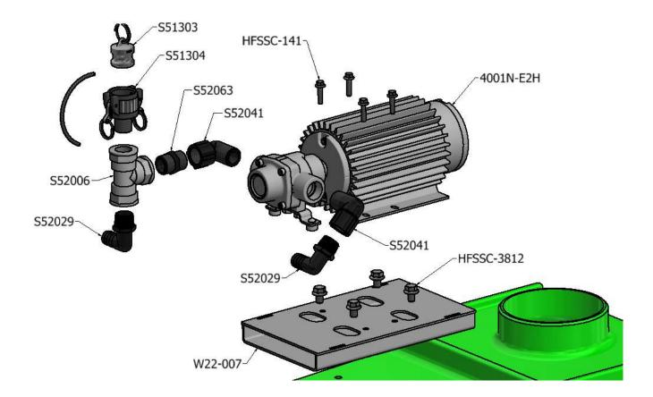
Back flush port / clean out. Can be used for prime.
