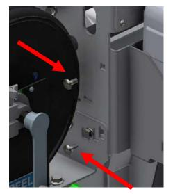
Attach the control valve assembly to the side of the upright using (2) 3/8 X 1" carriage bolts provided with the kit and reuse the nuts that were removed.
