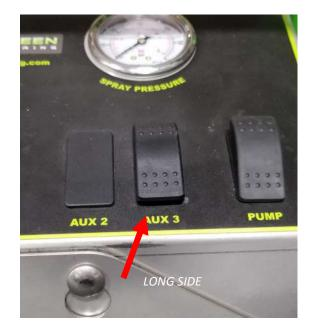
Plug the wiring harness into the rocker switch.
