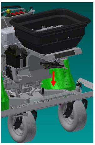
**STEP FIVE:** Disconnect the hydraulic hoses from the circulation fitting and reconnect them to the hopper.
