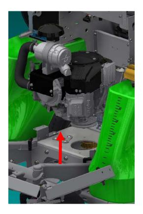
**STEP SIXTEEN:** Remove the engine pully and install it on the new engine.
