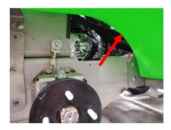
**STEP TWELVE:** Remove the heat shields from the chassis.
