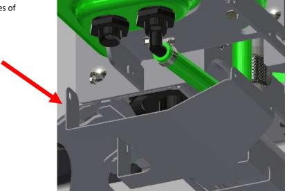
**STEP TWENTY:** Connect the "green" 1" X 16" hose to the inlet valve of the strainer & securely fasten with hose clamp.
