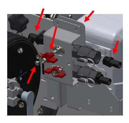
**STEP ELEVEN:** Remove the 3/4" elbow fitting from 35 gal. tank suction port & install the 3/4" X 1" elbow provided with the kit (EL100 HB).
