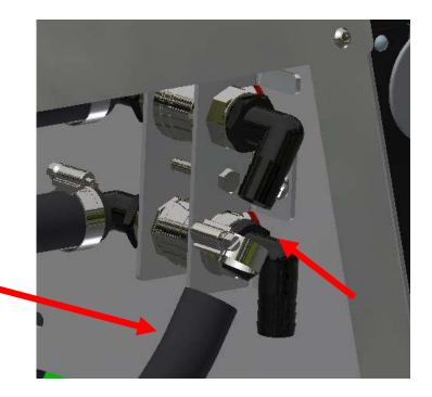
**STEP SEVEN:** Loosen the hose clamps & remove the suction hose from the strainer to the suction line.
