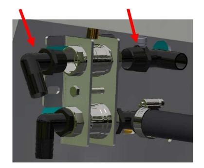
**STEP FORTEEN:** Loosen the hose clamp & remove the suction hose from the strainer "outlet" port.
