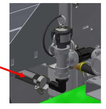
**STEP SIXTEEN:** Remove the fittings from the strainer and install the 3/4" X 1" barb fittings provided with the kit (S52017).
