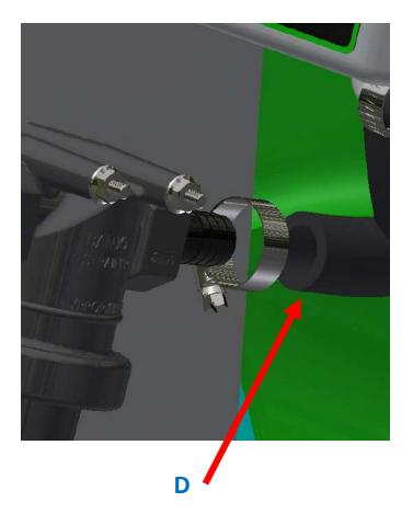
**STEP FIFTEEN:** Loosen the hose clamp & remove the suction hose from the pump "inlet" port.
