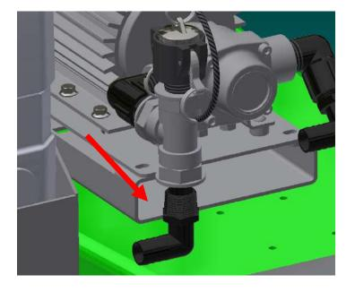
**STEP EIGHTTEEN:** Install the 1" suction hose assembly provided with the kit to the suction valves & securely fasten with hose clamps.
