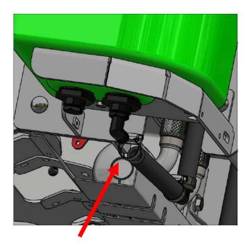
**STEP THREE:** With the drip pan still in place, Loosen the hose clamp from the suction hose and remove the "drop hose" assembly.
