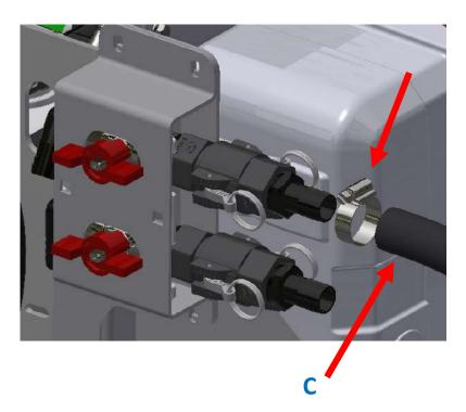
• Loosen the hose clamp & remove the suction hose from the 35 gal. tank suction.
