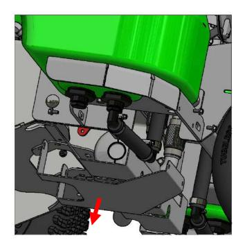
**STEP TWO:** Loosen the hose clamp and disconnect the suction hose.
