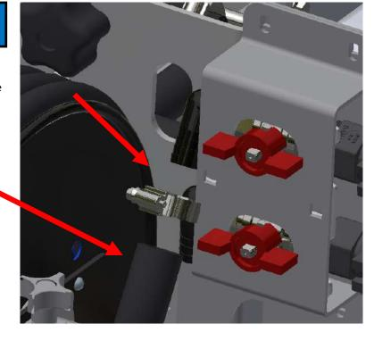
• Loosen the hose clamp & remove the suction hose from the *quick disconnect* valve.
