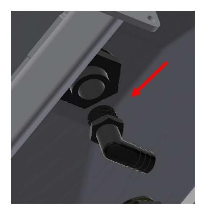
**STEP TWELVE:** Loosen the hose clamps on the left & right suction valves and remove the 3/4" suction hose assembly from the suction valves.
