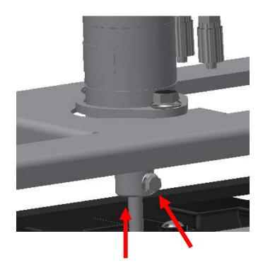
**STEP TWO:** Place a bucket under the hopper trap, open the trap to drain the hopper.
