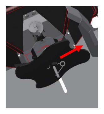
**STEP TWO:** Slide the spinner off of the rod.
