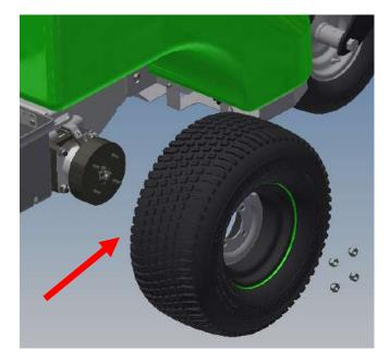
**STEP TWO:** Locate and remove the rubber tab on the inside of the hub.
