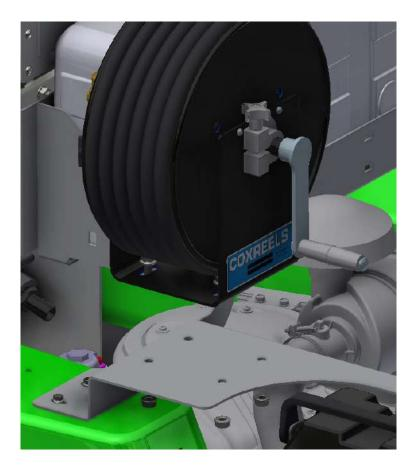
**STEP SEVEN**: Install the barb fitting (S52021) to the bulkhead fitting above the fuel tank.
