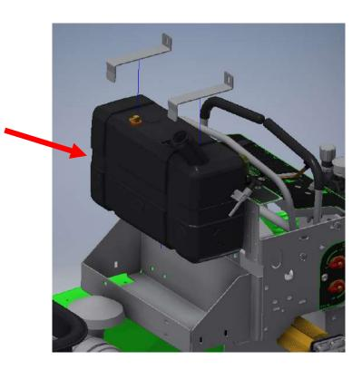
**STEP FOUR:** Attach the hose reel mounting bracket.
