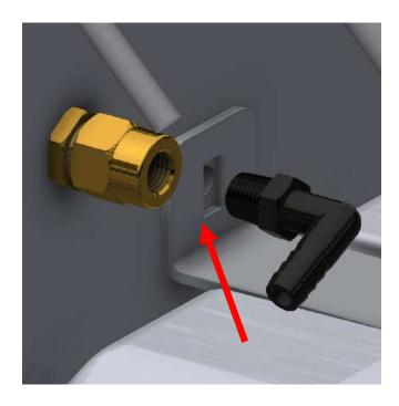
**STEP EIGHT:** Attach the 3/8" hose (S55005) to the hose barb fittings and securely fasten with (2) 3/8" hose clamps (MS4).
