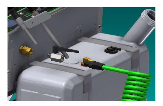
**STEP THREE:** Disconnect and remove the fuel tank.
