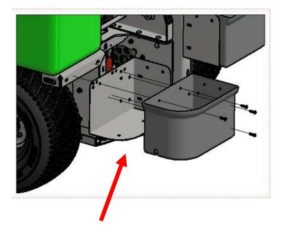
**STEP THREE:** Install the supplemental tank to the frame as shown.
