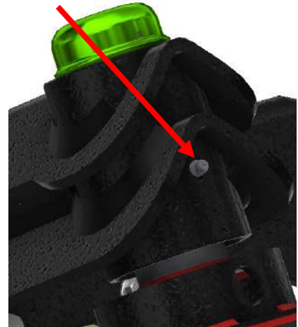
Castor Tube Grease Point (BOTH SIDES)
