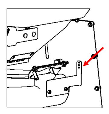
**STEP TWO:** Remove the deflector cable from the dash panel.
