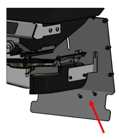
**STEP FOUR:** Drill two mounting holes in the left side panel as shown.
