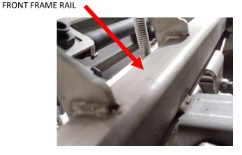
Remove the bolts in the frame and attach the plow hitch to the frame. Repeat the process for the right side.
