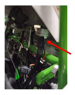
**STEP 33:** Connect the "fused" connector to the positive terminal on the usb port.
