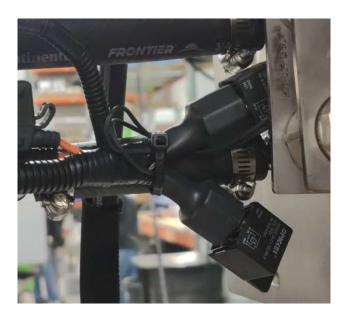
**STEP 30:** Route the wires for the foot switch down the upright with the existing bundle, through the hole in the foot board and connect them to the foot switch.
