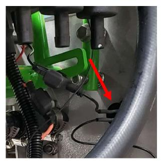
**STEP 34:** Connect the #9 ground wires to the upright cross member.
