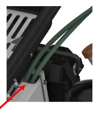
• Connect the hoses from the plow hitch to a the *right side (LIFT)* of the control valve.
