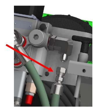
• Attach the other end of the hose to the hydraulic pump. (*end with 90° fitting*)
