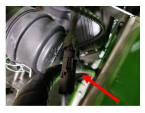
**STEP TWELVE:** : Once all hose connections and wiring connections are made, securely fasten the wiring harnesses to the frame with zip ties and wrap hoses with protective rubber hose wrap.
