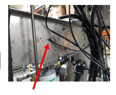
**STEP ELEVEN:** Plug the pump power connector from the harness to the foam marker power connector.
