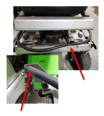
**STEP SIX:** Cut the provided hose to length as needed and route it from the "tee" fitting, along the frame, and connect it to the foam marker pump.
