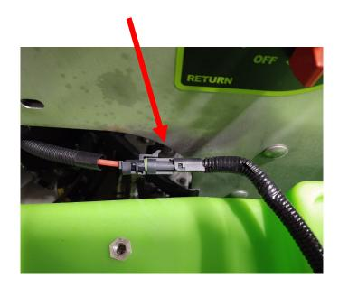
**STEP THERTEEN:** Reconnect the battery, *power* wire first along with pump harness power wire and then *ground*.
