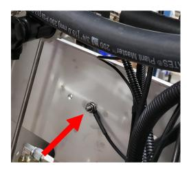
**STEP TWELVE:** Connect the pump plug from the harness to the pump.
