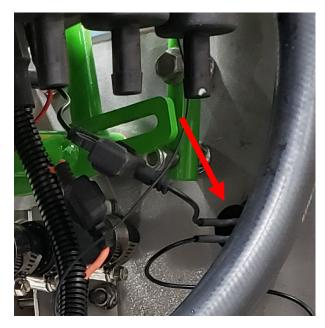
**STEP ELEVEN:** Connect the lower ground wire to the up right cross member.
