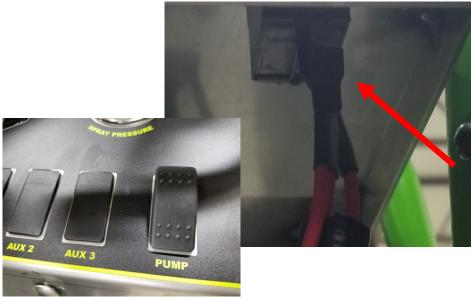
**STEP NINE:** Connect the ignition plug to the ignition switch on the dash panel.
