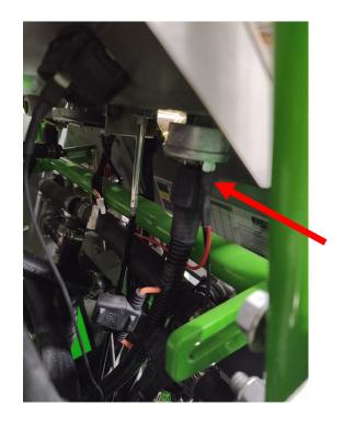
**STEP TEN:** Connect the "fused" connector to the "usb" port.
