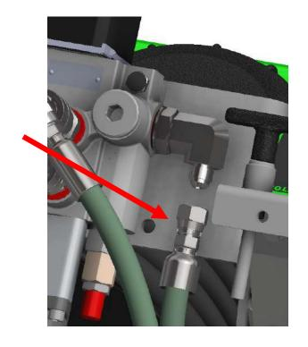
Attach the other end of the hose to the hydraulic pump. (end with 90° fitting)
