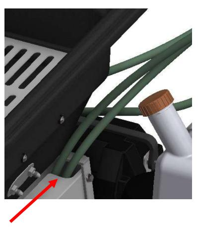
Connect the hoses from the snow plow to left side (ANGLE) of the control valve.
