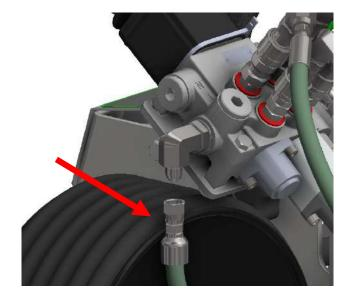
Attach the other end of the hose to the input port of the hopper control valve. (end with 90° fitting)
