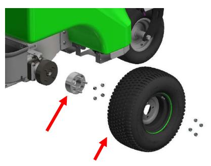
4 Remove the front tires and install the 13" front tires provided with the kit.
