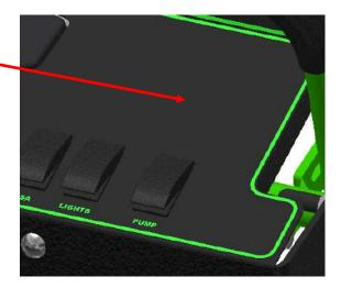
• Once the opening is exposed, attach the switch (provided with the kit) to the dash.
