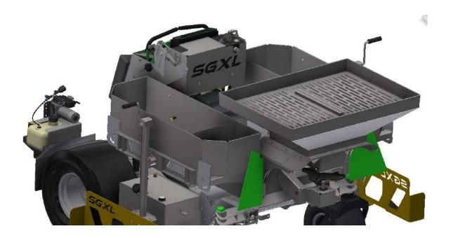
• With the help of a second person, lower the hopper onto the frame. Be sure the holes are lined up with the hopper and the frame.
