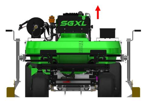
• Once the spray system is clear of the frame, back the machine out from under it.
