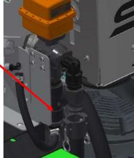
Disconnect the relief tube from the push-lock fitting.
