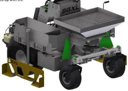
• Attach the bolts securing the hopper to the frame.
