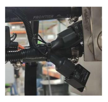
**STEP 30:** Route the wires for the foot switch down the upright with the existing bundle, through the hole in the foot board and connect them to the foot switch.
