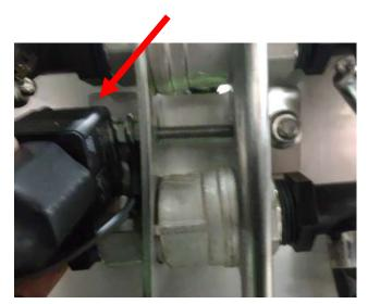
Secure the relay end of the harness to the suction hose with zip ties.
