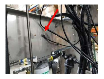
**STEP 35:** Connect the red power wires to the engine solenoid.
