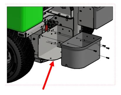
**STEP 3:** Install the supplemental tank to the frame as shown.
