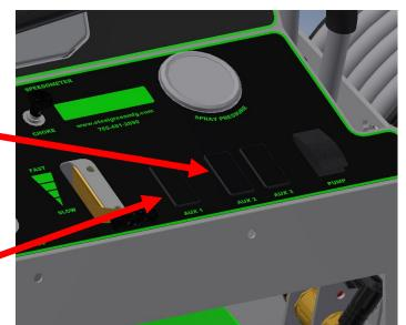
**STEP 5:** Attach the rocker switch to the appropriate opening.
