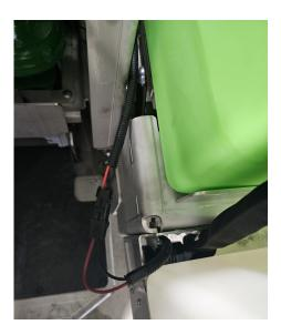
**STEP 10:** Reconnect the battery *power wire* first along with the *pump power wire* from the wiring harness, and then reconnect the *ground* wire.
