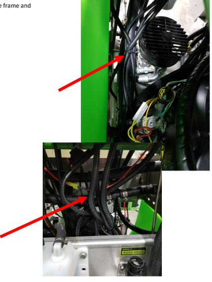
**STEP 7:** Connect the wiring harness to the rocker switch.
