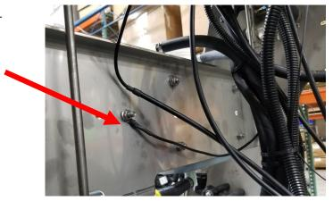
**STEP 9:** Connect the plug on the harness to the pump on the 7 gallon tank.
