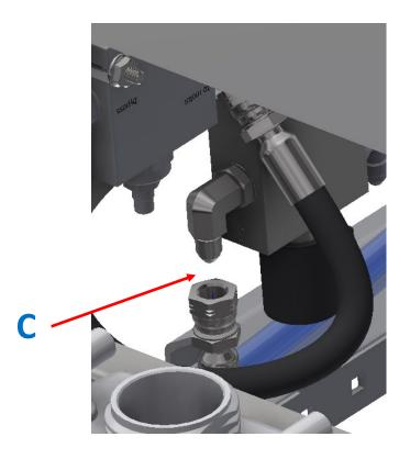
Connect the other end to the tee fitting on the hydraulic pump.
