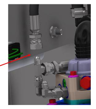
• Connect the elbow end of the 1/4" x 14-1/2" hose to the supply tee fitting on the hopper control valve.
