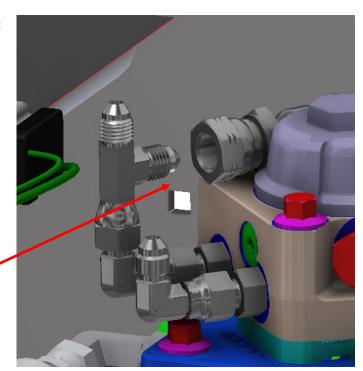
• Connect the elbow end of the 1/4" x 13" hose with to the return tee fitting on the hopper control valve.
