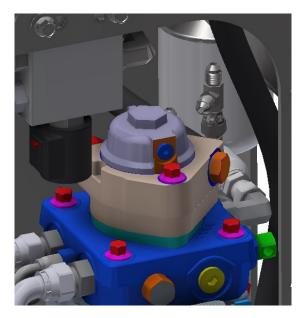
Loosen & reposition the elbow fittings as shown.
