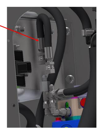
Disconnect the supply hose from the hydraulic pump.
