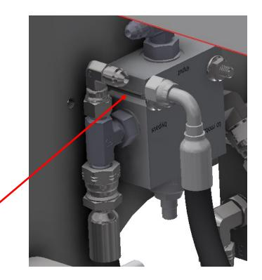
Connect the other end to the tee fitting on the hydraulic pump.
