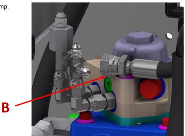
• Disconnect the other end at the hsa valve & remove the hose.
