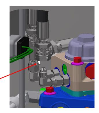
Connect the straight end of the 1/4" x 7-1/4" hose to the hopper control valve & the elbow end to the hsa valve
