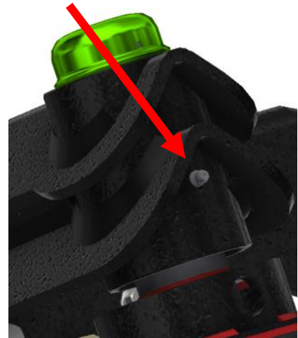
CASTER TUBE GREASE POINT
