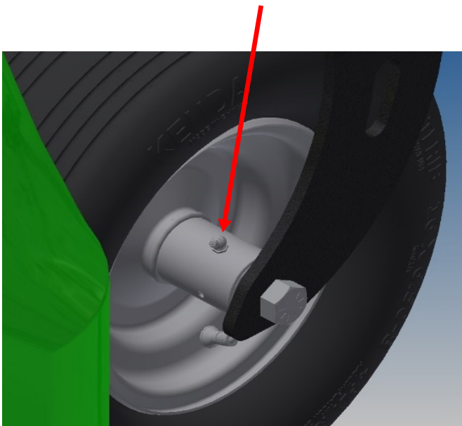
FRONT TIRE GREASE POINT (BOTH FRONT TIRES)
